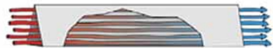
Traditional catalyst element – straight-line laminar flow: Most exhaust gas never contacts the catalyst.
